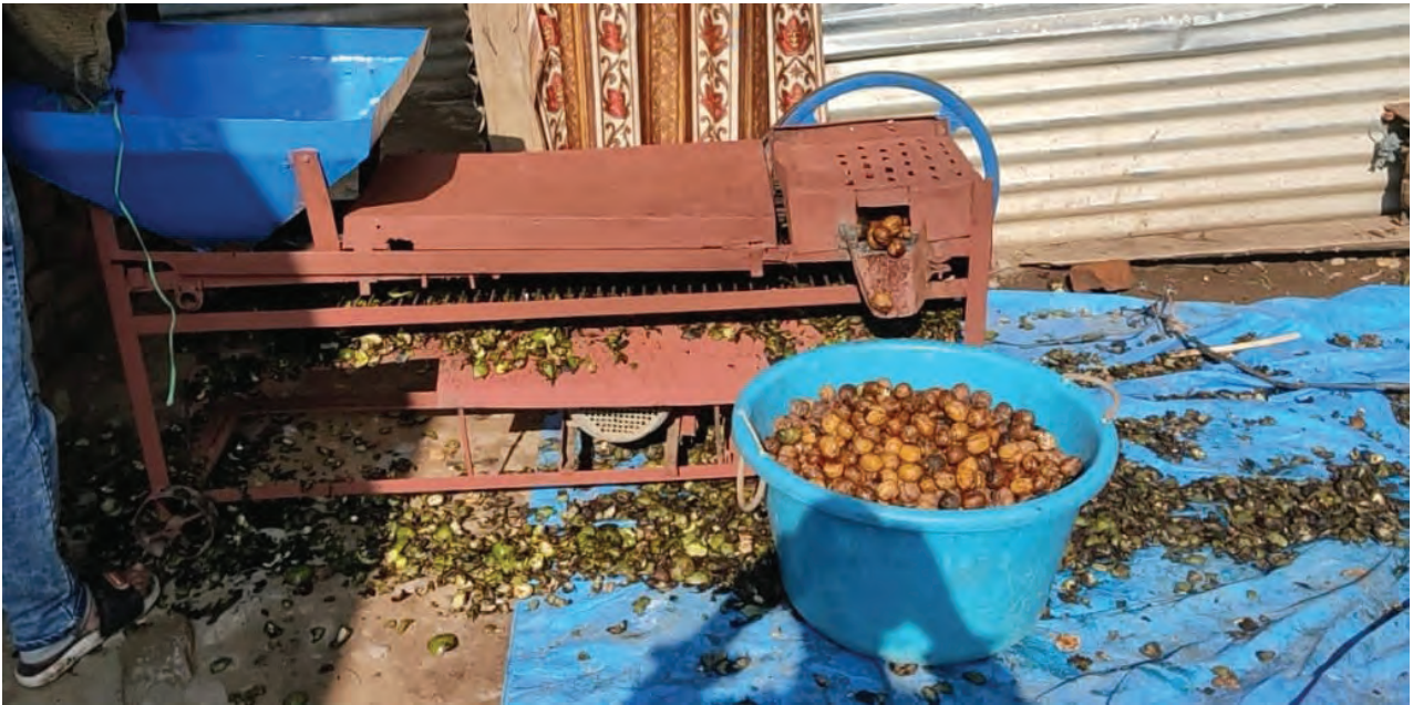
Walnut Peeler, an innovative technology scouted from J&K (UT) and subsequently value added has significant application in food process industry
