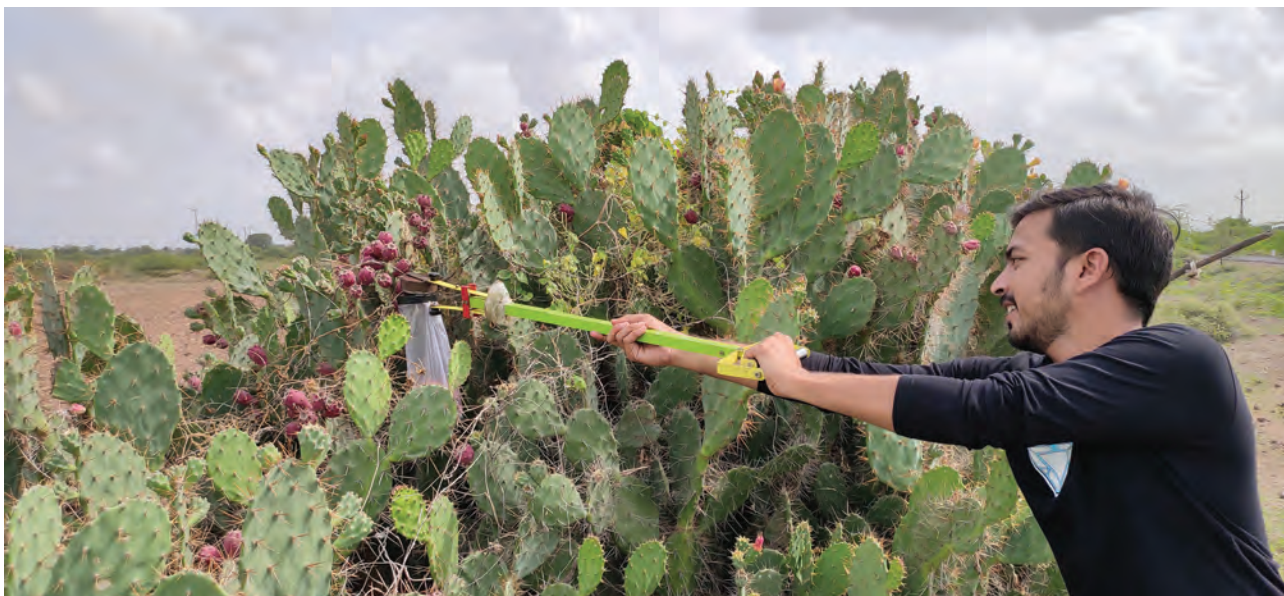
The Cactus Fruit Picker is an innovative technology which assist farmers in plucking of fruits surrounded by pointed spines
