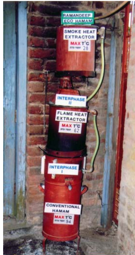
The Raman Deep Eco Hamam (Water heater)
