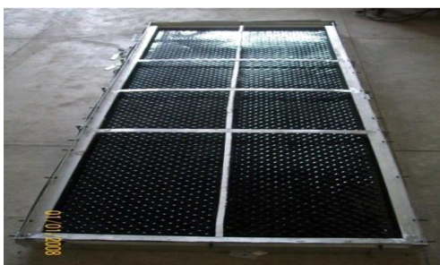
Fig.5 Improved Solar Air Heater Supervisor: Dr. Partha Praim Dutta, Associate Professor, ME, TU. Students: Jugal Saharia, Nayan Moni Sarma Design: Hemispherical Protruded Application: Efficient Hot Air Generation for Drying of Agricultural Crop
