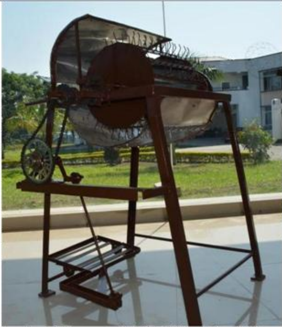
Fig.4 Manual Paddy Thresher Supervisor: Dr. Dilip Datta, Associate Professor, ME and Dr. Uddhab Bharali, Visiting Director, CIIE, TU
