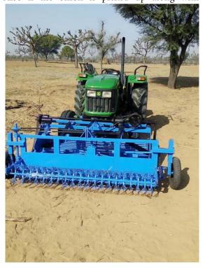
the leaves, separation of soil from the onion becomes a difficult job. In order to mechanize the process, Shrawan developed two machines; one for cutting leaves and another for digging, picking up and cleaning soil from the bulbs. Presently, he is trying to combine both the machines together as a unit i.e. as onion leaf cutter cum digger.
