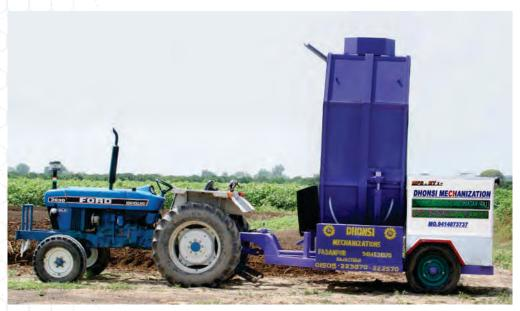
chopping into small pieces, mixing and lining the biomass. A hydraulic jack has been provided to facilitate the up and down movement of the rotor. At the side of the tractor, a water tank with 1500 liter capacity has been provided. This water is used to moisten the compost while the rotor blades are turning the heap of biomass. A weight box has been provided next to the water tank to maintain balance during movement.
