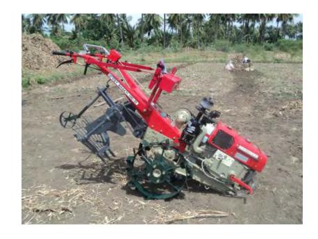
turmeric rhizome from soil without damage. It has a field capacity of about 0.2 acre per hour while consuming 1.5 liter of fuel (diesel). The cost of harvesting per acre almost comes to half if the present machine is used for harvesting and laborers are engaged for collection.
